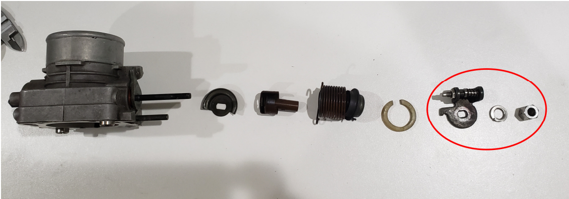
FIGURE 1 - disassembly of throttle body return spring mechanism
